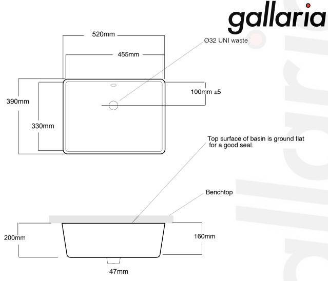
Fixing: No mechanical fixing supplied. Use Bench or Wall-mounted Tapware
